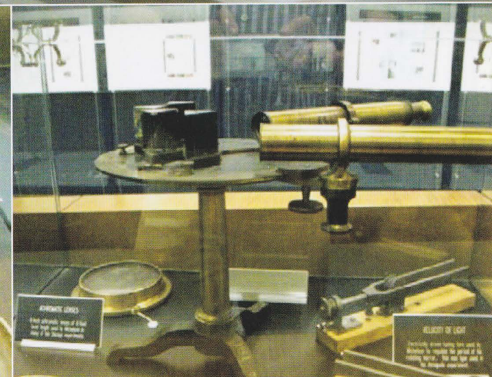
VELOCITY OF LIGHT Electrically driven tuning fork used by Michelson to regulate the period of his rotating mirror. This was type used in his Annapolis experiment.
