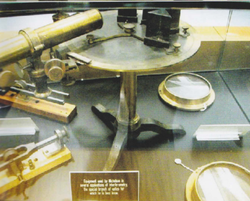
ROTATING MIRROR First rotating mirror of 8 inch diameter used by Michelson in several applications of interferometry.
